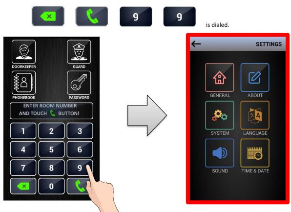
2. Entering SETTINGS if the device screen is button shape: Please press PASSWORD icon LONGER THAN 5 SECONDS.
