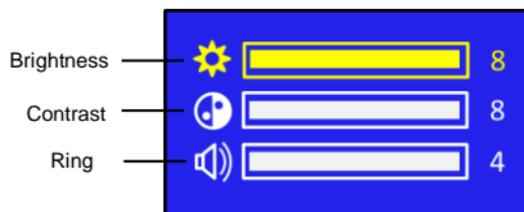
The brightness setting at the top of the first Menu screen has selected as YELLOW. You can change the value of the selected setting by using the + and - buttons under the menu button.
