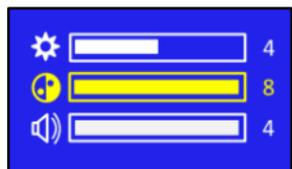
You must press the menu yer button again to switch to the Ring setting under Color. In this case, the "Ring" setting has selected as "YELLOW. You can change the value of the selected setting by using the + and - buttons.
