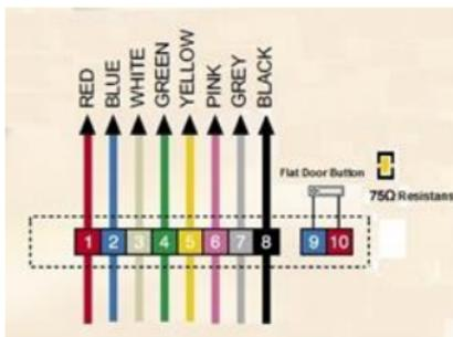
**Note:** When needed, please use the 75 ohm terminal jumper to terminate the intercom connection.
